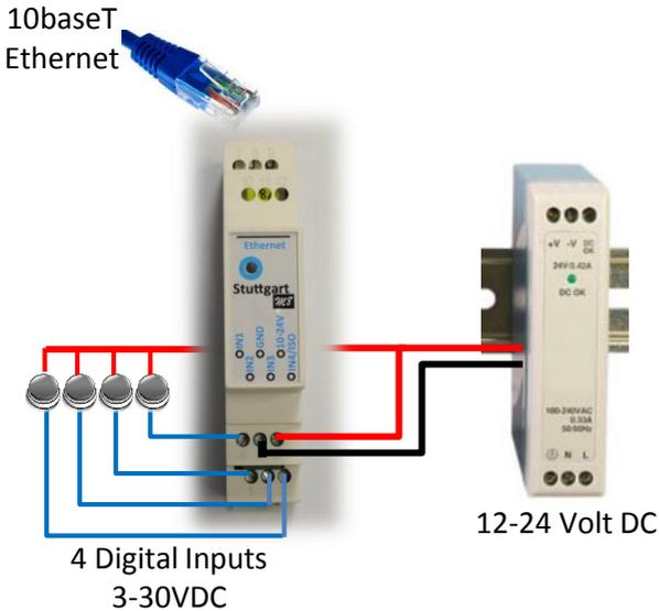
There are 4 Digital Inputs. A voltage present on the input will activate the input.
