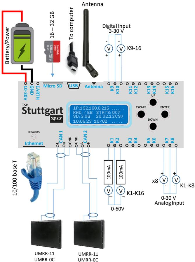
Take care in connecting the earth connector to chassis or earth ground. Internal Surge protection is provided from both the positive and negative terminal to this point and any surges will dissipate to that point.
