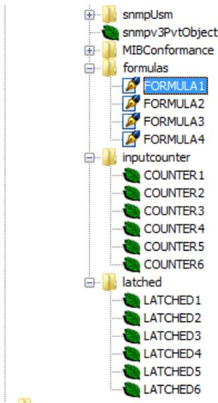
The Digital inputs are value 0 or 1. A value 1 indicate that a voltage of 3-40VDC is present on the digital input. INPUT1=D1 and INPUT6=D6. COUNTER1-6 indicate the number of level changes for the corresponding input. An upgoing edge on D1 will increment COUNTER by 1 and a downgoing edge on D1 will increment the COUNTER by 1. The maximum value for count is 65535 and at the next transition the value will roll over to 0.
